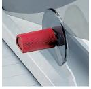
Variable clamping pressure can be applied with the manual hand clamping device.
